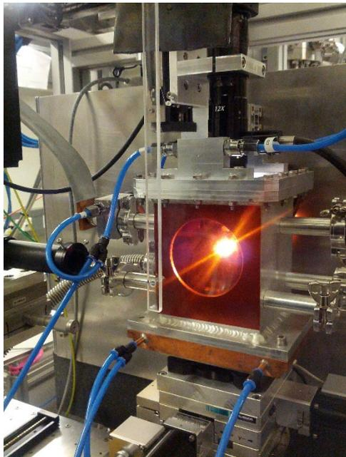
*Figure shows experimental setup for high-pressure/-temperature experiments on CaSiO<sub>3</sub> at the Extreme Conditions Beamline P02.2 at DESY, Germany.*
